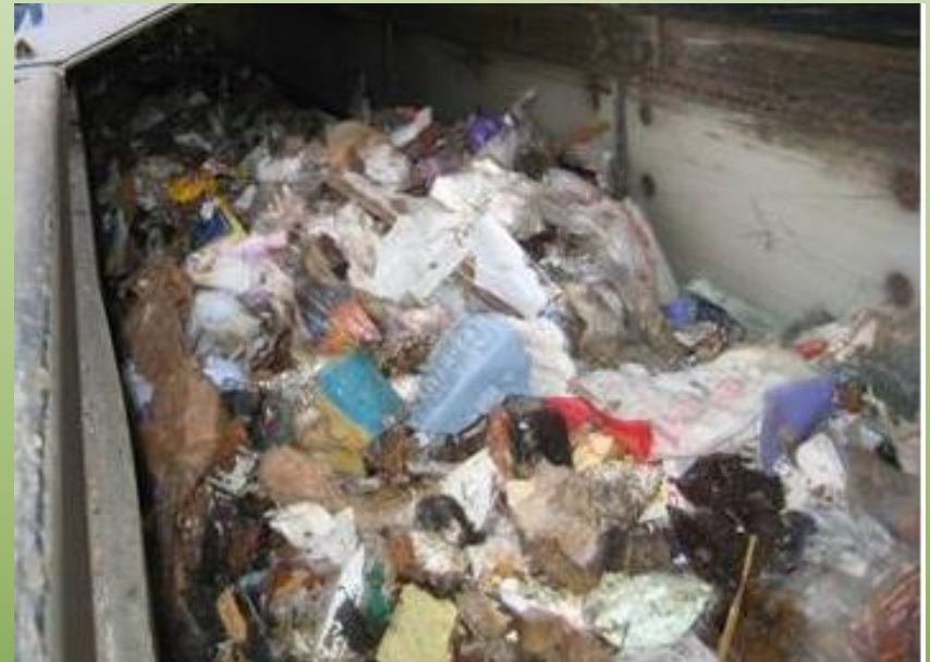
Minimally prepared "black bag" waste on GPRS™ input conveyor in Ottawa
